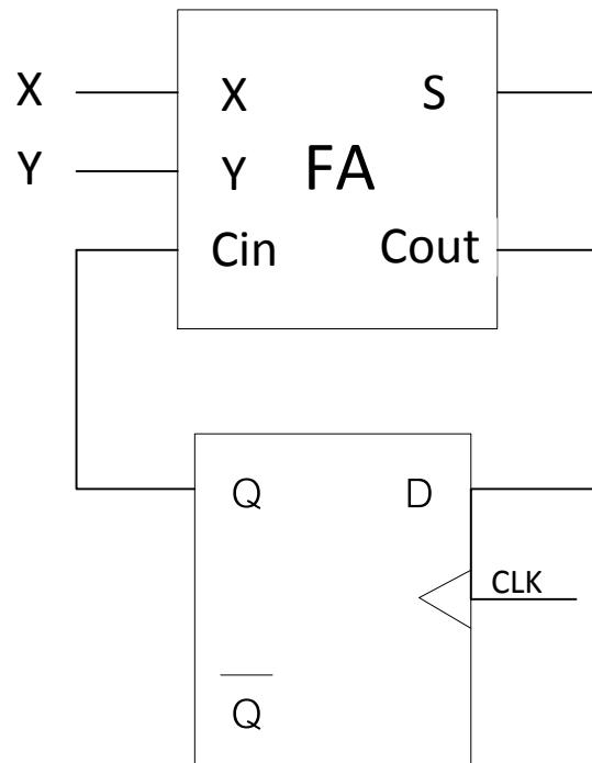
5) Counter design. Show all steps. Design a counter with the following binary sequence: 0, 1, 3, 7, 6, 4 and repeat. Use D-flip flops
